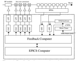
Figure 1. Fast feedback system schematic.
