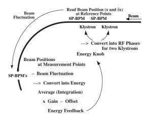
Figure 1: Process flow for beam-energy feedback.
