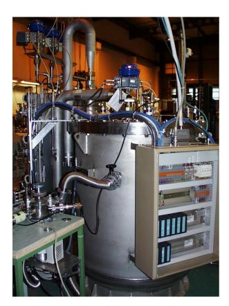
Figure 2: overview of the cryostat and remote I/O
