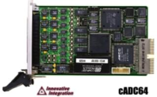
Figure3: The CompactPCI I/O card, from Innovative Integration, with a TMSC32 DSP on board.
