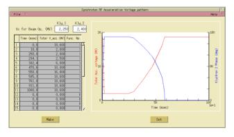
Figure 3: RF acceleration voltage ramping pattern editor window.
